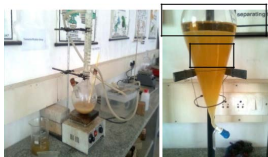
Figure: scum, Methanol & acid mixture and Separation of FFA layer
