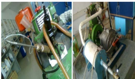
Fig: Kirloskar Diesel Engine with sensing exhaust gas temperature
